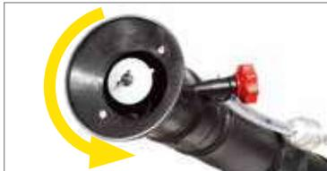
The opening angle of the jet can be adjusted rapidly and conveniently without having to stop working, enabling treatment to be customised according to each individual type of vegetation.
