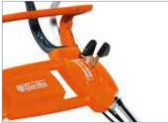
Model **VK** is equipped with stepless traction control so that ground speed can be adapted continuously to match the needs of the job.
