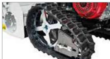
Propulsion system with oscillating tracks that adapt to various types of terrain (**TR** models).
