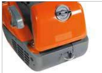
Snap hook: fold-away steel snap hook for rapid attachment of the tool to the operator's harness.
