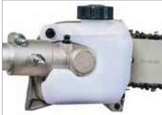
The semi-transparent chain oiler reservoir enables the operator to read the oil level without removing the cap. The oil pump with automatic delivery is adjustable, allowing the oil flow to be varied according to the use and the type of wood.
