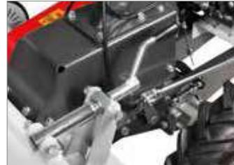
Cutting height adjustment by means of a worm screw lever. Finely adjustable from 20 to 80 mm.
