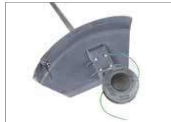
Ø 110 mm Tap&Go EVO line head, Ø 2.4 mm line, Tap&Go operation.
