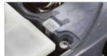
"Ice device": ensures the machine can operate without difficulty even at low temperatures (below 0°C), avoiding the formation of ice on the air filter.
