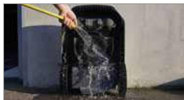
The **IPX5** rating (degree of protection against water) makes the robots a durable and reliable tool because they can be used even in the most difficult weather conditions. The cutting attachment can be washed directly.
