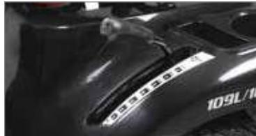
Practical cutting height adjustment with a conveniently positioned lever, with a graduated scale to show the cutting height at a glance.
