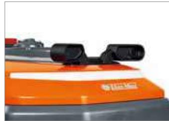
Ultrasonic obstacle detection to increase the performance and safety of the robot mower; the sensor (optional) can detect obstacles 10 cm wide and 15-20 cm high in front of the machine.
