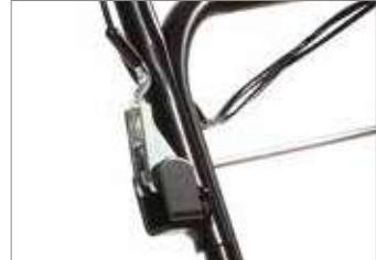
Simplified handlebar fold-down system:
