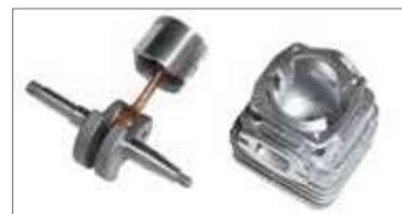
Piston with 2 rings, forged and machined steel crankshaft and connecting rod, needle roller bearings, nickel plated cylinder: high and constant efficiency guaranteed over time, even when undertaking heavy work schedules.
