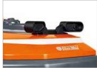
Ultrasonic obstacle detection to increase the performance and safety of the robot; the sensor (optional) can detect obstacles 10 cm wide and 15-20 cm high in front of the machine.
