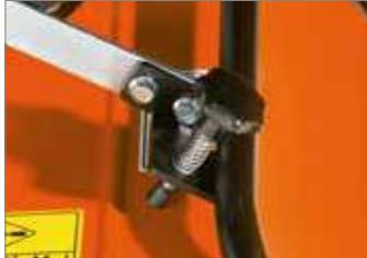
Working depth adjustment spring.
