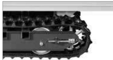
Rugged undercarriage with track tensioner sprocket, perfectly balanced for correct weight distribution and excellent grip on all types of terrain.
