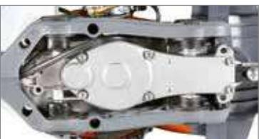
Anti-vibration system utilizing 4 springs guaranteeing total isolation from the operator's hands.
