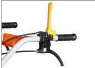
Handlebar-mounted gear lever.
