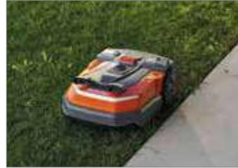
The robot mower cuts along the boundary wire first, in order to cut as close to the lawn edge as possible.
