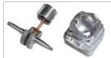
Piston with 2 elastic rings, forged and machined steel crankshaft and connecting rod, needle roller bearings, nickel plated cylinder: constant high efficiency guaranteed over time, even when undertaking heavy work schedules.
