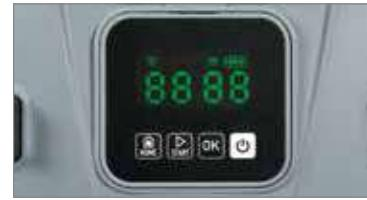
The digital LED display indicates what the robot is doing and enables faults to be easily eliminated by following the troubleshooting instructions in the app.
