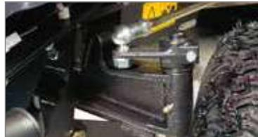
Front axle cast in steel to withstand even the heaviest of duties and resist accidental impact.
