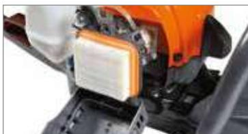
Large paper air filter for higher filtration capacity and more effective engine protection, even in dusty conditions.
