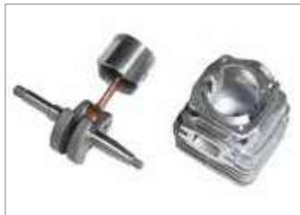
Piston with 2 elastic rings, forged and machined steel crankshaft and connecting rod, needle roller bearings, nickel plated cylinder: constant high efficiency guaranteed over time, even when undertaking heavy work schedules.
