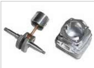
Piston with 2 rings, forged and machined steel crankshaft and connecting rod, needle roller bearings, nickel plated cylinder: constant high efficiency guaranteed over time, even when undertaking heavy work schedules.
