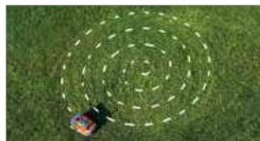
Spiral cutting can be used when mowing an area with tall grass: the robot keeps working in this mode until the grass is of equal height.
