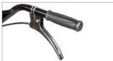
Centralised cutting height adjustment controlled by means of a handy lever located on the handgrip, affording maximum comfort for the operator.
