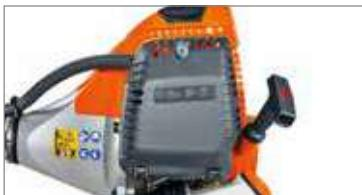
Filter cover secured with two screws, easily removable to facilitate maintenance.
