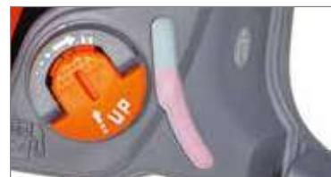
Fuel tank with externally visible level; easy management of refueling intervals.
