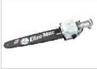
Cutting system: lightweight and compact, equipped as standard with a carving bar with sprocket tip. The guide bar measures 12" (30 cm) and is paired with a 1/4 x .043 chain.
