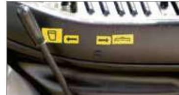
Mulch/collect “Change over” system: using a handy lever, the operator can close off the collection duct and switch automatically to mulching mode, without stopping.
